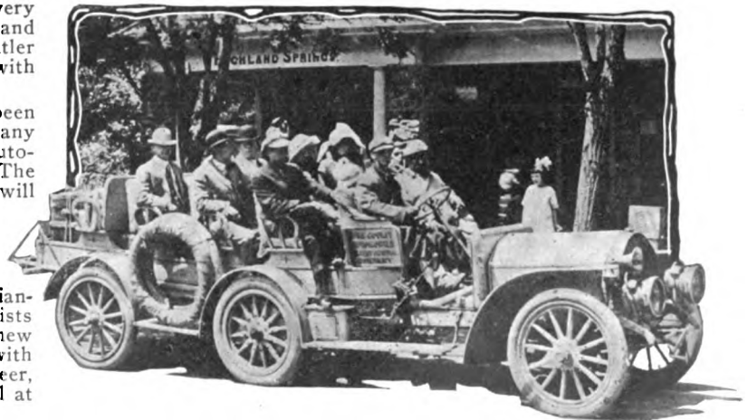
Six-wheel, fourteen-passenger, sight-seeing bus built by the Lake County Automobile Transportation Company, Highland Springs, Cal. The car used is a 7-year-old Columbia
